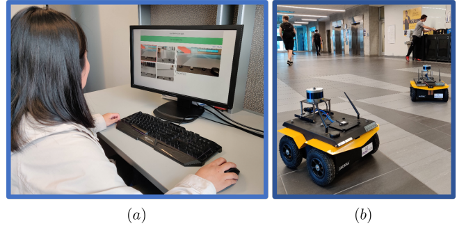
Fig. 1: Multi-robot supervision user study setup: a) A participant monitoring multiple robots using the web-based interface, b) Clearpath Jackal robots used for the study.
