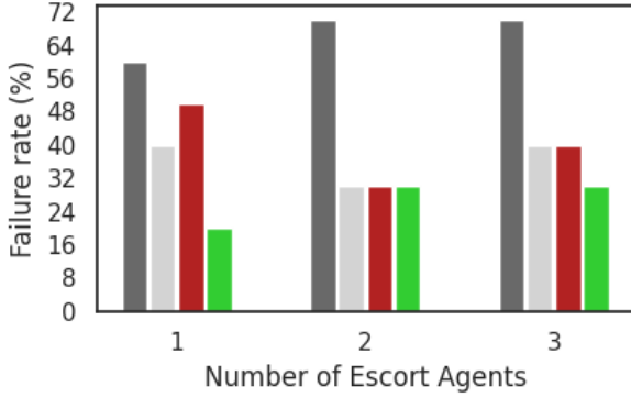
Fig. 3. PA's failure rate with different EA reward variants. Higher is worse. Failure is recorded when the PA collides with an object. Dark grey: blind, light grey: MI-UCB, red: SI, green: SE.
