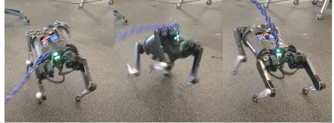
Fig. 1. Spirit’s spatial anchoring controller recovers from a strong rolling disturbance. The resulting perturbation is incurred while engaged in the energetic sagittal plane pitching required by the bounding gait. Despite the high adversarial velocity in roll, the anchoring controller enables the robot to regain its balance and resume stable bounding. The frames shown span approximately 600 ms and offer a visualization of the comparable recovery behaviors quantified in Table I.
