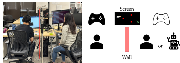
Fig. 4: Human-in-the-loop experimental setup, in reality (left) and in concept (right). For the Turing test, we purposefully block audio-visual observations of the partner from the human subject using headphones and a wall (shaded in red) separating both parties.
