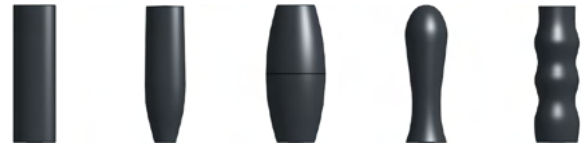
Fig. 9: Diagram of the selection of handle contours used for force-torque characterization. The contour line has been parametrized as a curve defined by a quadratic polynomial. The coefficients of the polynomial are randomized within a bounded range to generate a cross-section which is subsequently revolved around a central axis to generate the handle model.
