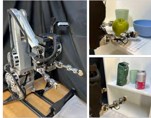
Fig. 1. Manipulation platform with reflexes for autonomous grasping. Our reflexive grasping controllers utilize our manipulation platform’s high-bandwidth actuation and low-latency sensing modalities to perform autonomous grasping tasks, such as clearing a cluttered shelf.
