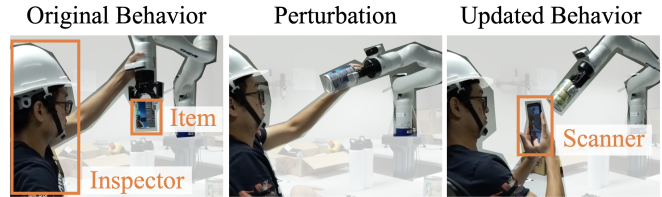
Fig. 1: OPA interprets human feedback in relation to specific objects, enabling fast online adaptation. In this scene, the default behavior (left) is to carry a can upright to a dropoff zone. After a perturbation in orientation (middle), the robot learns to hold the can correctly, allowing the human inspector to scan its label properly (right).
