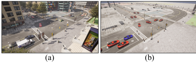
Fig. 6. (a) Traffic scene at busy intersection in Carla, ego vehicle blue on the left; (b) The same scene in the Digital Twin recreated using the object list data. Note that vehicle types are not distinguished at this stage.
