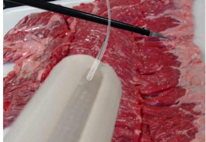
Fig. 1. An example of robust image segmentation for a concentric tube continuum robot. The robot is successfully identified, as illustrated by the white overlay, despite the presence of multiple, partial occlusions and a background of similar color.
