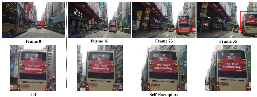
Fig. 1. It is ubiquitous that relevant content can be found in a long time span in a video. Therefore patches with similar content but higher resolution can be found in other frames. These patches with higher resolution can be used as exemplars to super-resolve the LR patches.
