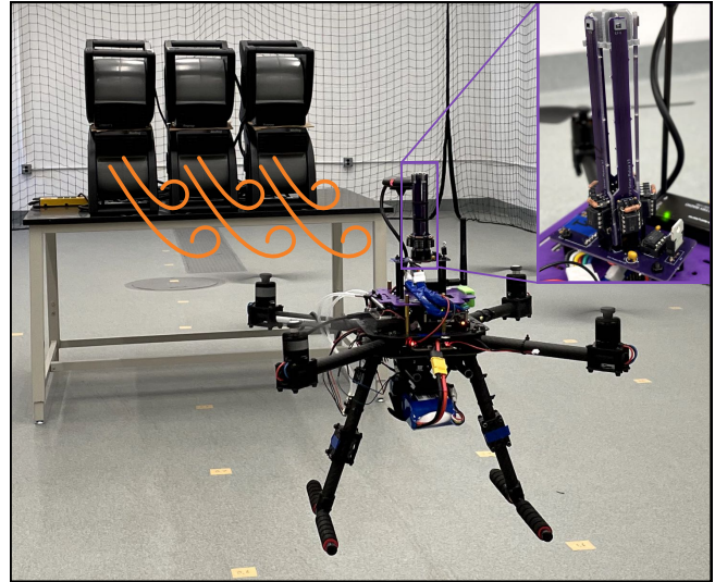
Fig. 1: FlowDrone incorporates the MAST (top right), an omnidirectional flow sensor leveraging MEMS hot-wires to provide fast and accurate estimates of in-plane wind magnitude and direction, enabling superior flight performance in windy conditions.
