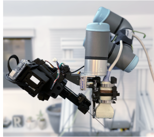
Fig. 1. Our Mechanical Ultrasound Scanning System, which consists of a linear array ultrasound transducer attached to the end-effector of a 6-DoF Universal Robots UR3e serial manipulator.
