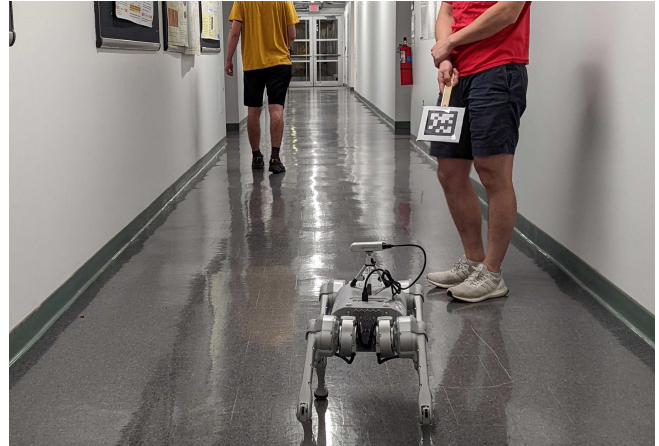
Fig. 1. A robot dog is tasked with following one of two humans that has a “treat” (the AprilTag [7] held by the human wearing the red-shirt on the right). The robot observes the state of the two humans (the x and y distances from the robot), infers which human to pay attention to and therefore which to ignore, and then receives the reward of treats if it moves close enough to the human and maintains proximity. The humans can decide to switch who has the treat at any point, and the robot will subsequently need to switch its attention. Note that the robot is not tracking the AprilTag (which may be invisible at any given point in time), but rather the human who is inferred to have the treat.
