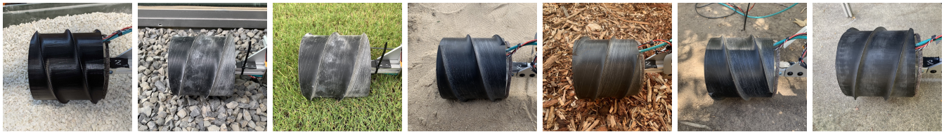
Fig. 3. Representative images of the test bed experiments conducted in the following media (from left to right): small gravel, big gravel, grass, sand, wood chips, dirt, and concrete.
