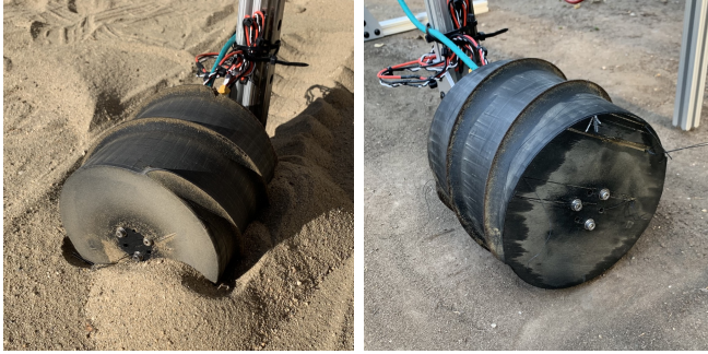
Fig. 6. When applying a 12N axial load during the sand and dirt experiments, the screw dug itself into the material. For the sand experiment (left), this caused slippage on the test bed's linear axis motor leading to inconsistent measurements. In the dirt experiment (right), the screw dug itself into a rock bed hence resulting in the screw slipping and leading to inconsistent results. Therefore, for both of these environments, we used a lower axial load of 6N in the linear motion experiments.
