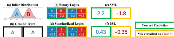
Fig. 3. Motivation of BSL. Suppose we have Class A and B with inlier distribution \mu_A = -2, \mu_B = 2, \sigma_A^2 = \sigma_B^2 = 1 before standardization in (a). Now consider the classification of two pixels with ground truth (b) of class A. The produced binary logits (c) are similar for the two classes but standardized logits (d) are quite different. As a result, Standardized Max Logits (e) yield anomaly scores with a drastic difference, which can lead to serious false positives. Blended Standardized Logits (f), on the other hand, smooth the anomaly score on pixels with higher uncertainty and alleviate false positives due to misclassification.
