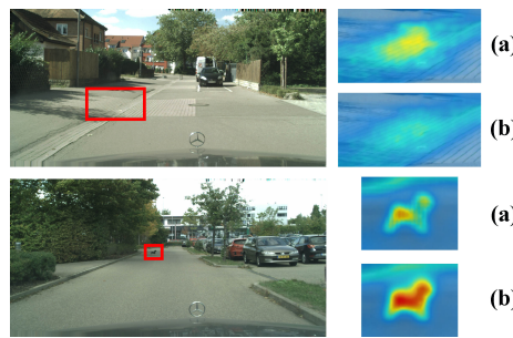
Fig. 8. Qualitative comparisons on different inference scales. (a) indicates using only the original scale while (b) indicates using multiple scale inference. Other configurations are aligned. Multi-scale inference can mitigate the unexpected false positive existing in a specific inference scale (the false positive region of the sidewalk in row 1) and can better identify distant obstacles (row 2).
