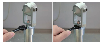
Fig. 2. Manually screw the target bolt. The principle of side screwing is similar to that of manual wrenches.
