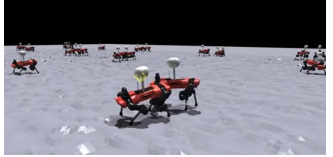
Fig. 5: Simulation environment for tracking the impact point \mathbf{p}_{\text{imp}} . The agents try to track the yellow spheres with the simulated nets mounted on their base, while avoiding the robot from falling in the presence of random pushes, randomized friction, mass and terrain.
