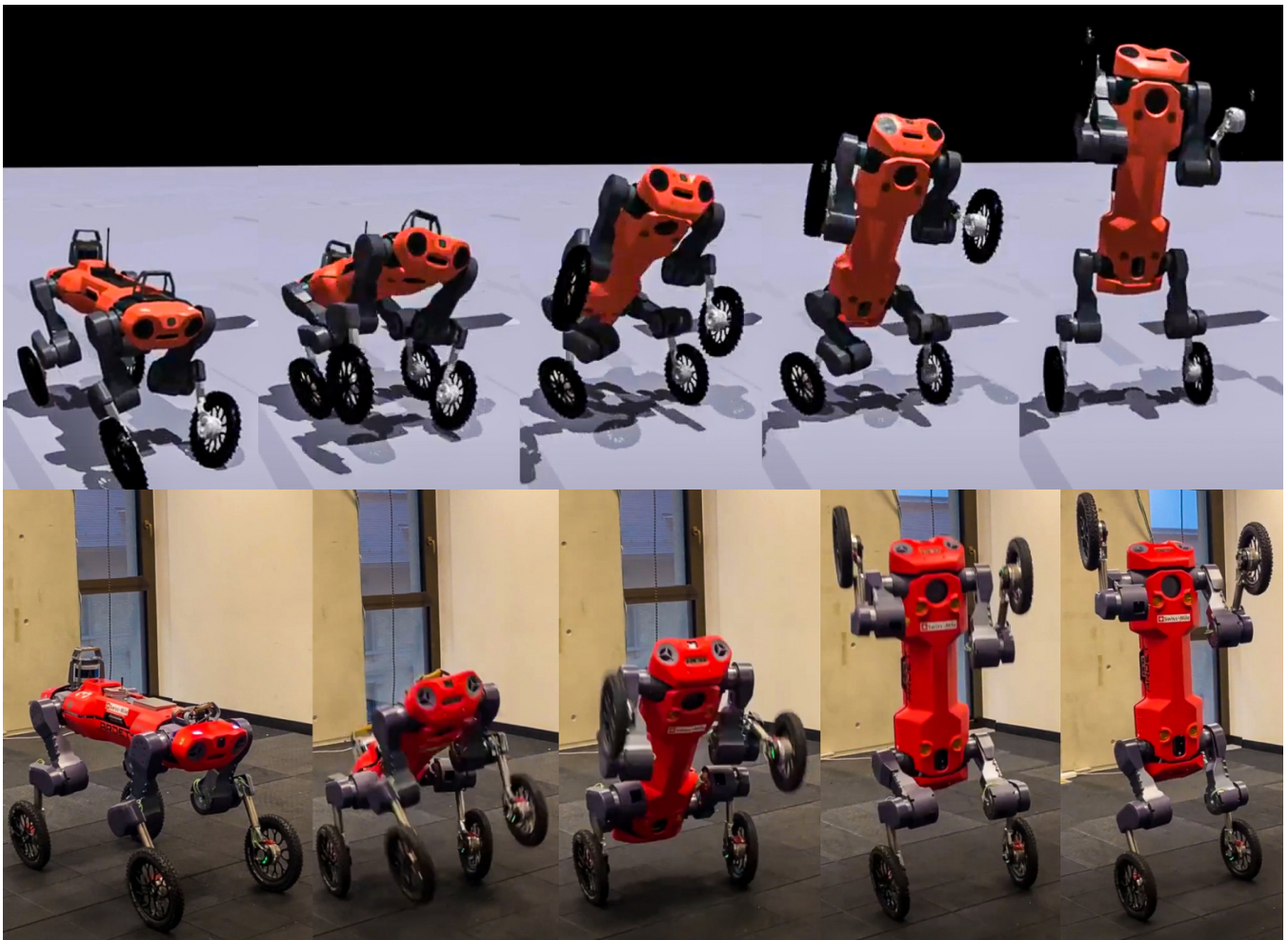
Fig. 4. Stand up-sequence in simulation and on the real robot. The policy is able to stand up, navigate large distances on two legs, and finally sit down again using motion data from the reversed stand-up sequence.
