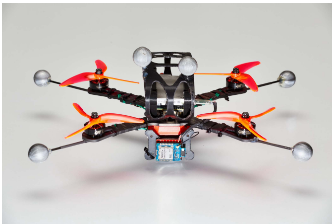
Fig. 12. Quadrotor platform that is used for real-world experiments. The achievable TWR is 4. The platform is equipped with a Laird module for real-time wireless communication, off-the-shelf components, and reflecting markers for the VICON localization system.
