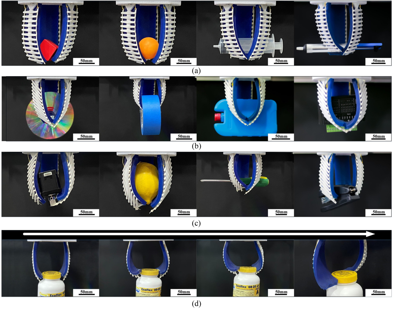
Fig. 10. Grasping performance of the gripper in the different attitude. (a) Grasping a wood square piece, ping-pong ball, injector (26.5 g), and glue straw in the attitude that the scaffolds of fingers 1, 2, and 3 are perpendicular to the spine. (b) Grasping a video disc, packaging tape (253.2 g), plastic box, and stepper motor driver in the attitude that the scaffolds of fingers 1 and 2 are not perpendicular to the spine, while finger 3 is perpendicular to the spine. (c) Grasping a stepper motor (374.1 g), lemon, screwdriver, and stapler in the attitude that the scaffolds of fingers 1, 2, and 3 are not perpendicular to the spine. (d) Unscrewing a bottle cap.
