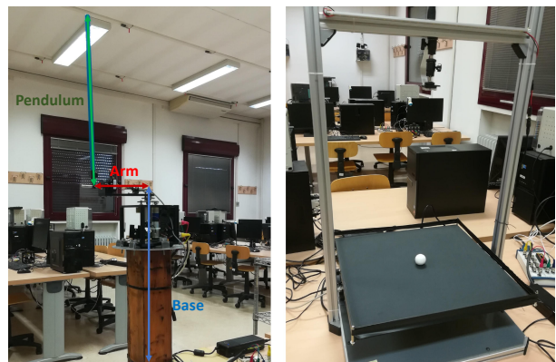
Fig. 12: (Left) Furuta pendulum controlled in the upward equilibrium point by the learned policy. (Right) Ball-and-plate system.
