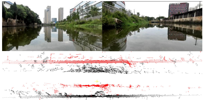
Fig. 8. A negative pair in sequence N03_2. The left figure and black points denote a frame, right figure and right points denote another frame. PointNetVLAD and NetVLAD mistakenly identify the negative pair as positive pair, but our method does not mistakenly identify them.
