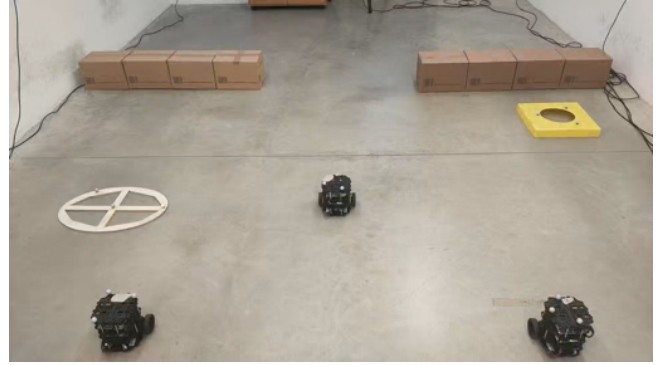
Fig. 6. Experimental setup utilized for the shared control of a multi-robot system. There are two obstacles, that the robots need to avoid, and a bottleneck the robots need to pass through.
