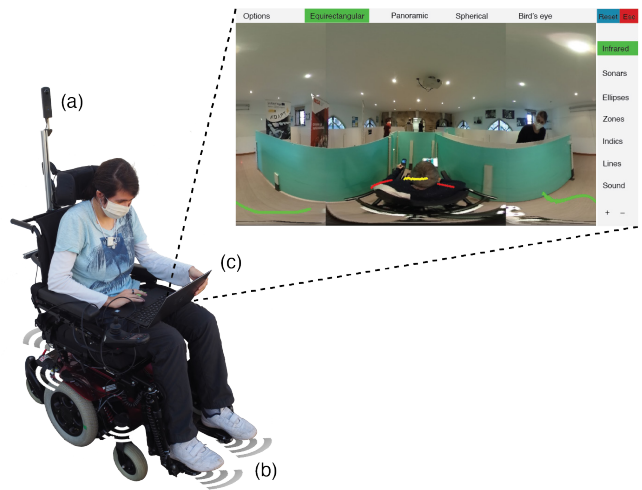
Fig. 6. The basic system components of SpheriCol. (a) Twin-fisheye camera, (b) wheelchair equipped with a ring of ToF sensors, and (c) user interface displaying a panoramic image of the surrounding environment, with coloured distance markers overlaid.
