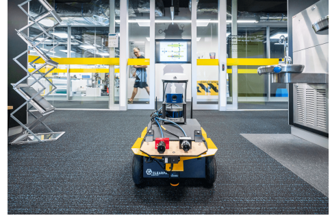
Fig. 4. Recording setup for the QCR-Event-VPR dataset. A DAVIS346 event camera (in red) was mounted on a Clearpath Jackal mobile robot. The camera can be installed forward-, side-, or downward-facing.
