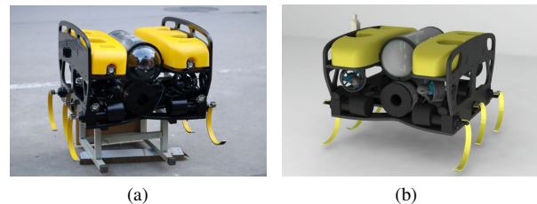
Fig. 1. The hybrid underwater hexapod robot. (a) The experiment platform. (b) The 3D model of HUHR.
