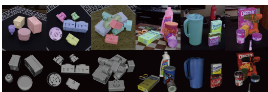
Fig. 6: The qualitative result of multi-object pose estimation. The first row represents the estimated poses and the second row is the reconstructed scenes using 3D object models on the T-LESS and YCB-Video dataset.
