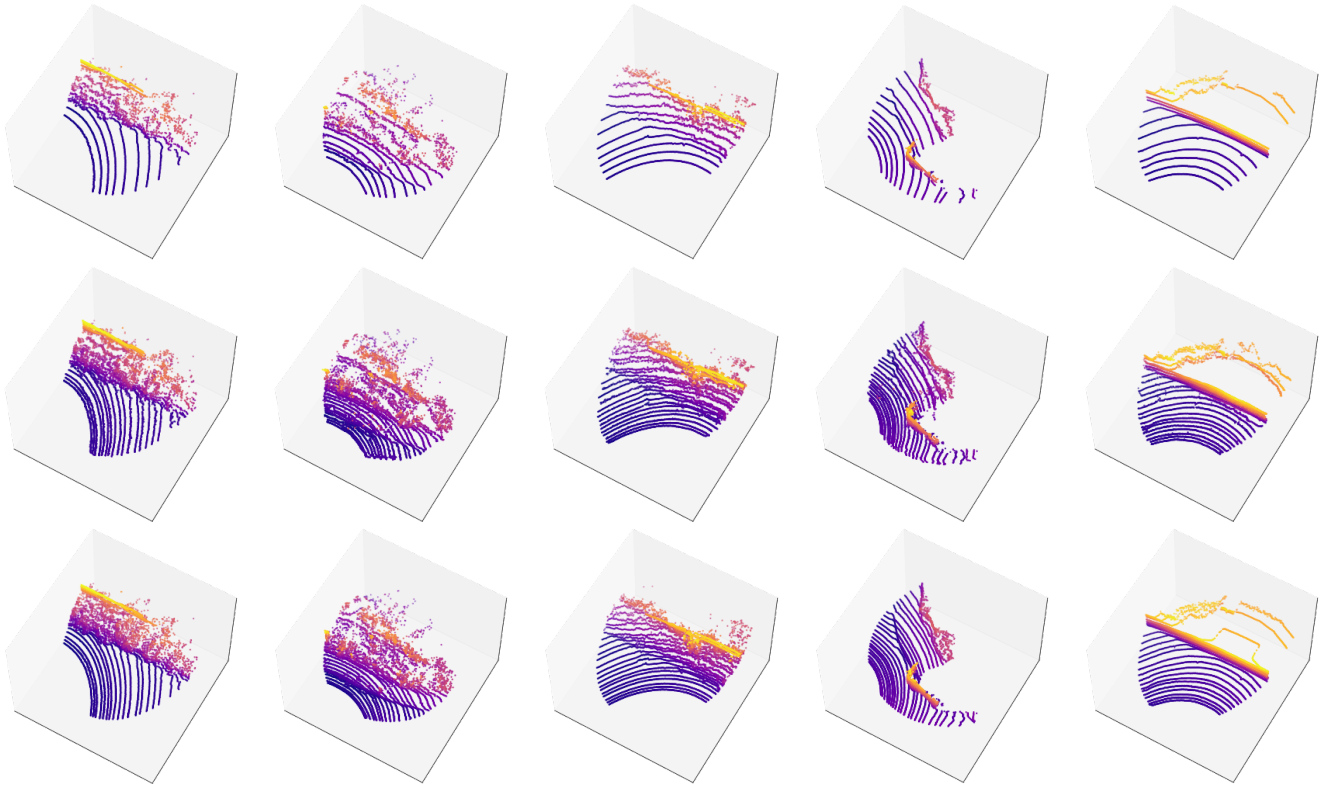
Fig. 8: Lidar upsampling results (middle) on KITTI val patches with input samples (top) and ground truth (bottom).
