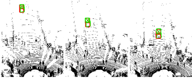
Fig. 9: Visualization in a sparse scene. The green box represents ground truth, and the red box represents the tracking result. In this scene, the target car ID is 63 in scene 4 of the KITTI dataset. The number of points for the target car is about 20.
