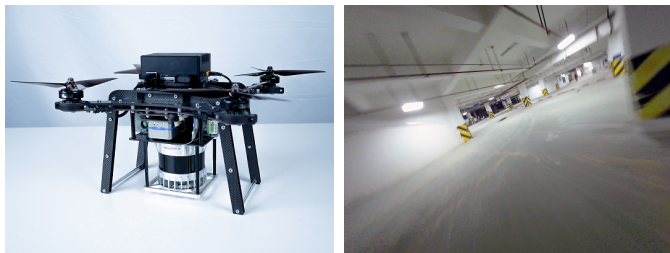
(a) Hardware settings of the vehicle. (b) An onboard camera image.
