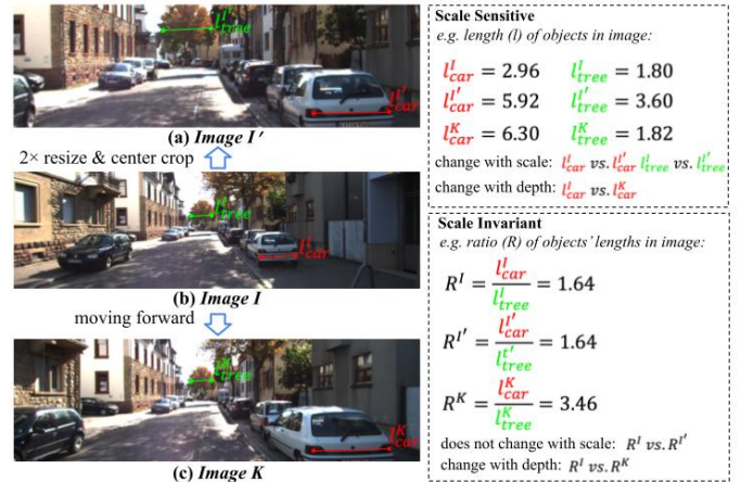
Fig. 1. Illustration on the influence of scale changes to the features. Image I' is an enlarged version of Image I imitating the scene captured by the camera with a larger focal length from the same viewpoint, and hence the depths of the same object in both Image I and Image I' should be the same. While Image K is captured after the camera moves forward from Image I , the depths of the same object in Image I and Image K are different.
