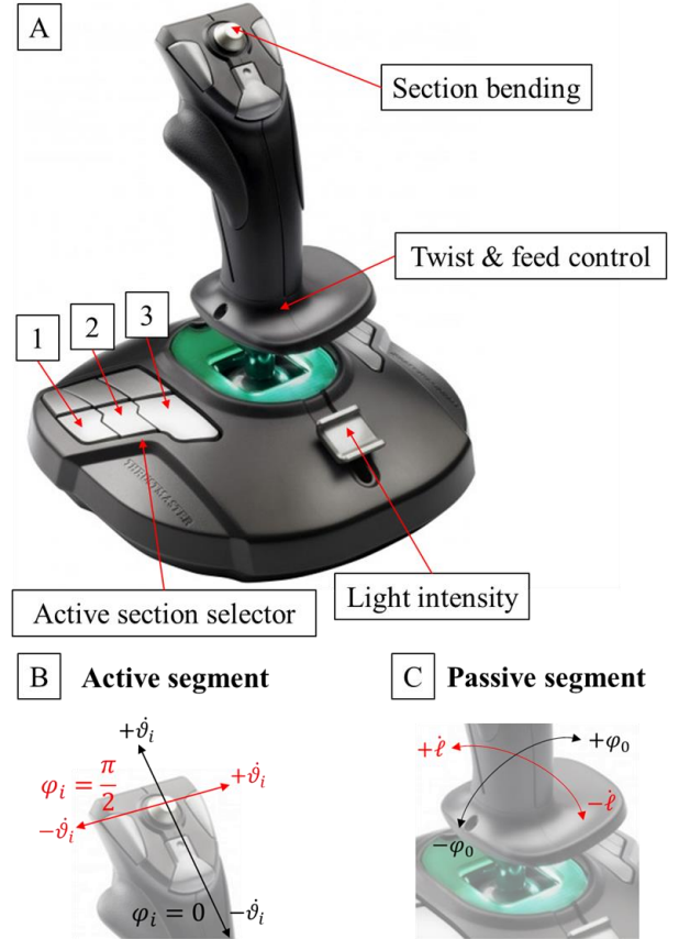
Figure 7. Controller mapping: a. Motion parameters of the continuum robot and corresponding buttons and joysticks on the controller; b. Motion variable mapping for the active segment, with control over the bending speed and direction; c. Motion variable mapping for the passive segment, with control on twist angle and feeding speed.
