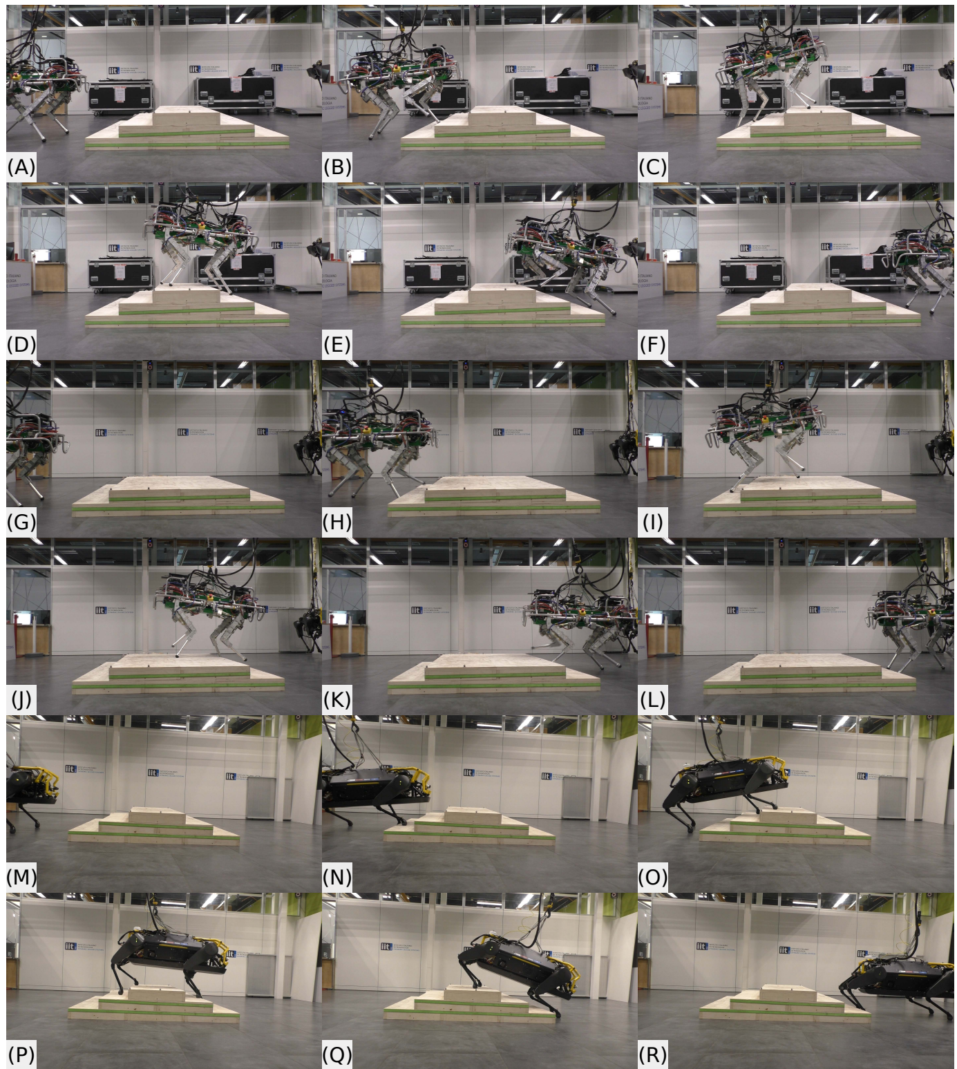
Fig. 6. HyQ and HyQReal climbing stairs in experiment. (A-F) HyQ crawling over with 0.1 m/s commanded forward velocity. (G-L) HyQ trotting over with 0.25 m/s commanded forward velocity. (M-R) HyQReal crawling over with 0.2 m/s commanded forward velocity.
