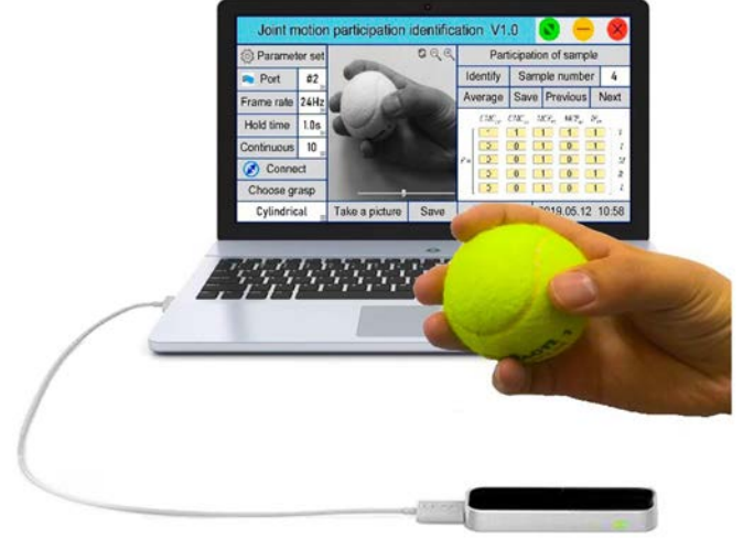
Fig. 2. Human hand motion acquisition system based on Leap Motion.
