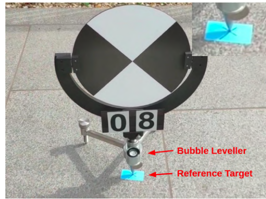
Fig. 8: A reference target placed on the ground and used for point cloud fine registration. Sparse ground truth points were created by placing Phasma at the cross-hairs of the reference target.
