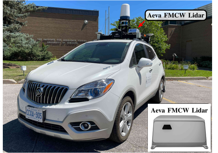
Fig. 5: Our platform, Boreas , is previously used to collect the Boreas dataset [40] and additionally equipped with an Aeva Aeries I FMCW Lidar [34] for use in this work.
