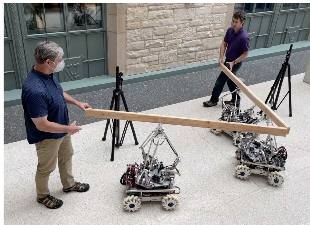
Fig. 10. Two humans and three Omnids manipulating a jointed payload.
