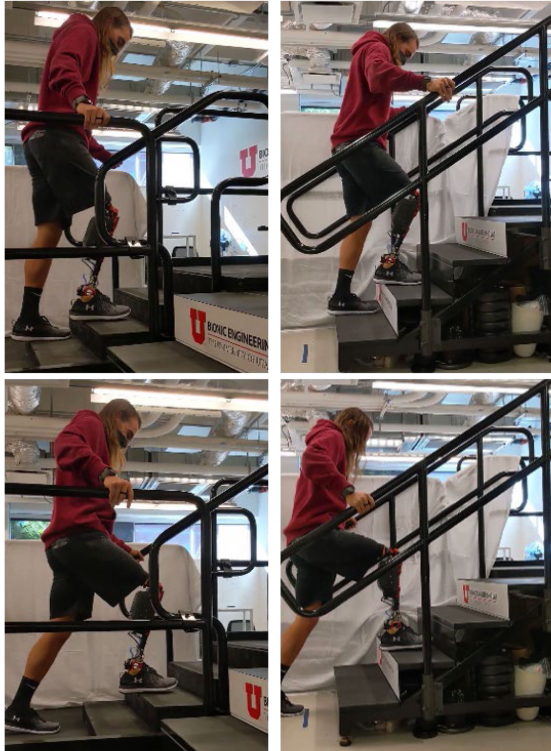
Fig. 4. Subject climbs stairs with the Utah Lightweight Leg. 4-in stairs on the left, 7-in stairs on the right. Step-by-step and step-over-step gait patterns are shown on top, two-step gait pattern is shown on the bottom.
