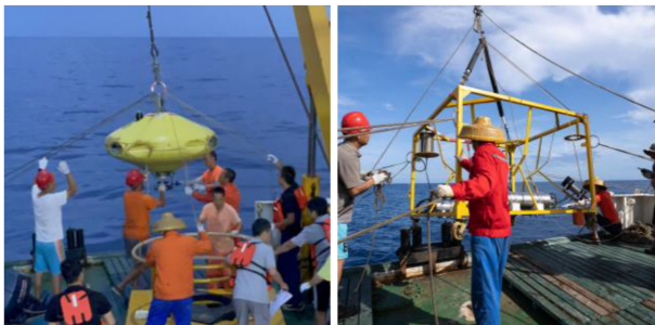
Fig. 14. Photograph of the G-AUH ( left ) and the subsea base station ( right ) to be deployed into the sea, taken on the R/V YueZhanYuKe-3 during the cruise in September 2021. Our piUSBL receiver and the acoustic beacon are respectively mounted on the G-AUH and the subsea base station.
