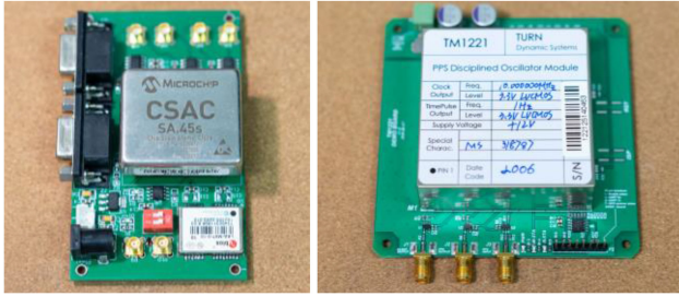
Fig. 2. Left : a commercial clock module with a Microchip Sa.45s CSAC. Right : a PPS disciplined oscillator module with an OCXO.
