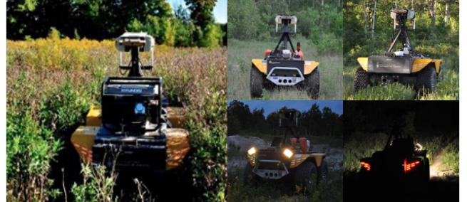
Fig. 1: Grizzly ground robot autonomously repeats a taught path with learned features despite severe lighting changes.
