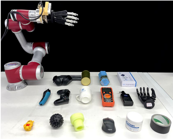
Fig. 8. Real-world experiment setup. The objects from top to bottom are headphone, cylindrical can, hexagonal prism, cardboard box, electric razor, gamepad, mug, multimeter, facial cleanser, prosthetic hand, cartoon model, massage ball, 3D printed object, mouse, cream box, electrical tape.
