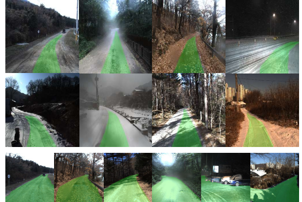
Fig. 1. We present a traversability estimation method that can be trained without human annotation in various environments. Top : Self-supervised traversability data gathered on diverse environments. There exists a large variance in visual appearances. Bottom : Traversability estimation results of the model learned solely with the self-supervised traversability labels.
