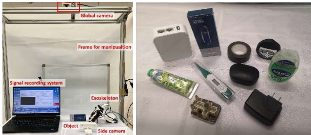
(a) Demonstrating platform (b) Grasping objects Figure 10. Demonstrating platform and grasping objects
