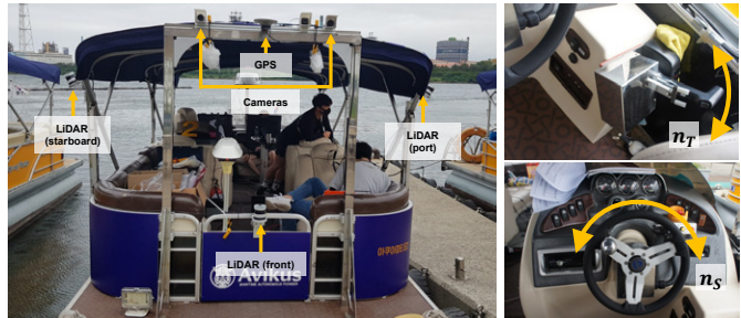
(b) Sensor configuration and thruster control devices
