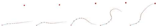
Fig. 14. Photo sequence of motion of end-effector regulation task on under-actuated serial manipulator. Red ball is the desired end-effector position with coordinates as [2.12, 2.12] m.
