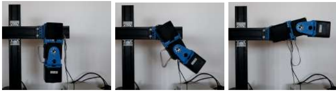
Fig. 3. Snapshots of the end-effector regulation task with the 2DoF system actuated by SEA in both joints. Please refer to the video attachment for more details.
