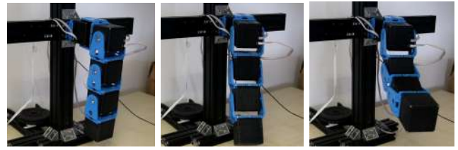
(a) Snapshots of the end-effector regulation for 4DoF with a SEA in each joint. Please refer to the video attachment for more details.
