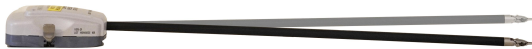
Fig. 3. Compliance of the surgical instrument. Similarly to backlash, this compliance is not reflected on encoder readings, and hence not reflected in the joint position estimation.
