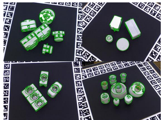
Figure 14. Qualitative results for T-LESS dataset, where the green edge line is a visualization of our predicted pose
