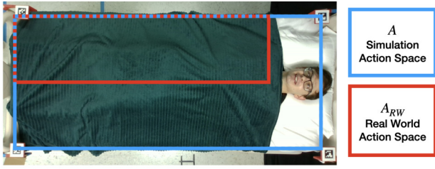
Fig. 5. Comparison of the action space used in simulation, A , and the action space used in the real world implementation, A_{RW} .
