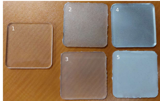
Fig. 4. The elastomers used in the comparative study: 1) Completely transparent, 2) Semi-transparent reflective, 3) Semi-transparent matte, 4) Opaque reflective, and 5) Opaque matte. It is important to note that membranes 1-3 are the focus of the study, while membranes 4-5 are not see-through and only used for comparison purposes in section III-C.
