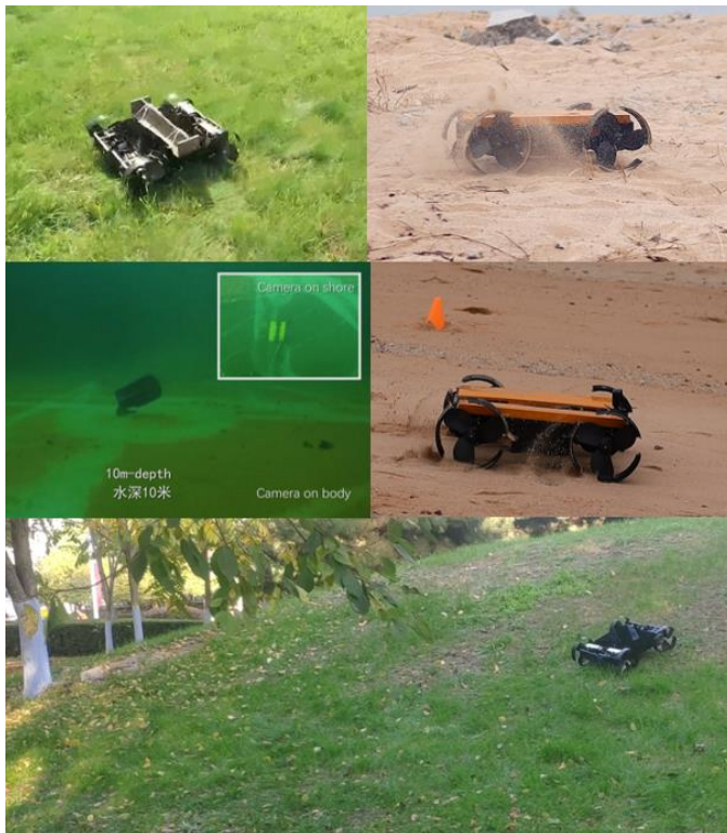
Fig. 16 The SHOALBOT successfully running over different challenging surfaces including turf, slope, dry sand, wet sand, and bottom of the pool (see video).
